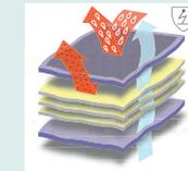
With 3 layers of melt-blown polypropylene in between 2 layers of spun bond polypropylene (SMMMS), the 4530 and 4530+ fabrics allow airflow, increasing breathability, reducing heat stress and improving comfort. The three melt blown layers are inserted with hot air and act as a barrier while the two outer spun bond layers make the coverall soft and breathable.
