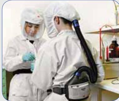
The modular respirator system is a comprehensive approach to worker protection systems based on comfortable-to-wear modules. All modular headtops, air delivery units and breathing tubes are compatible with one another. Users can mix and match parts as they move from one environment to another, or from one application to the next. It is the ultimate in flexibility for handling changing user environments.
