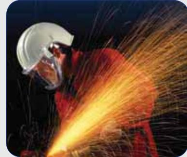
The individual respirator systems can be used in a variety of workplace applications. They include powered air respirators with integrated head, eye, face and respiratory protection and supplied air regulators with half and full face masks.
